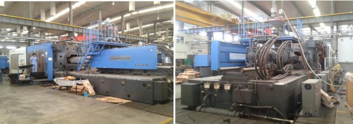
**Injection molding machine retrofitting model:** HTF2800X/1
