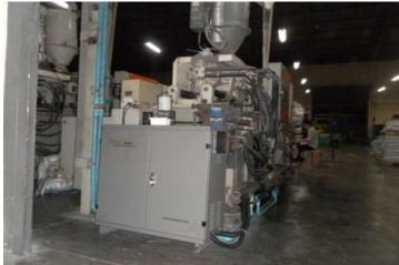
**Injection Molding Machine retrofitting** model:VICTOR Ve-140 **Molding product: fixed parts**
