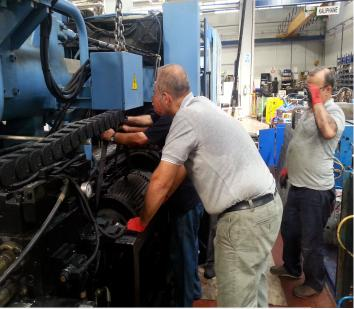
Injection Molding Machine retrofitting model: HTF530X
