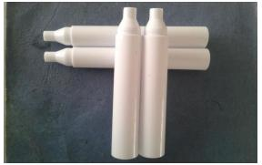
**Injection molding machine retrofitting** Model: HTF150X/1 **Molding products: pen** Molding material: PP Cycle time: 33.4s **Test Time: one week**
